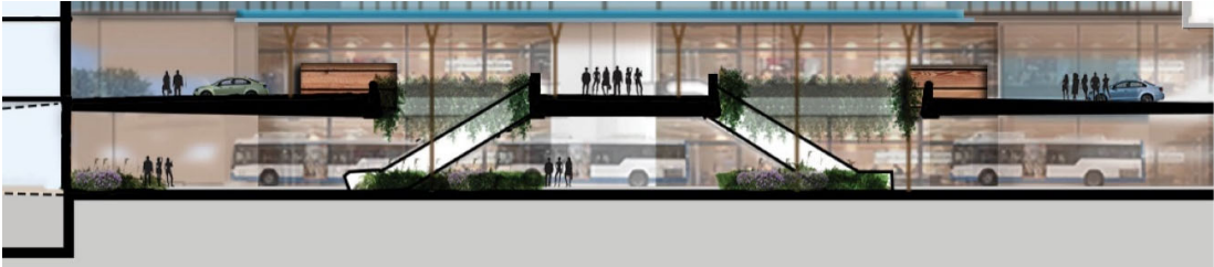
Figure 7 – Section diagram showing the new laneway on the upper level, with sunken south-bound bus terminus below
